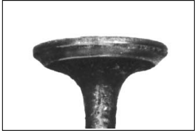
Stem Corrosion: Moisture in fuel or from condensation are the most common causes of valve stem corrosion. Condensation occurs from improper preservation during storage and when engine is repeatedly stopped before it has a chance to reach normal operating temperatures. Replace corroded valves.
